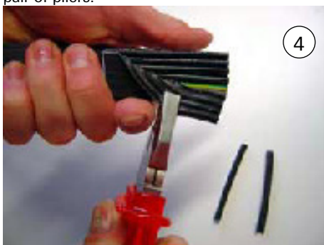
Tear the cable cleanly from below along the transverse scratch.
