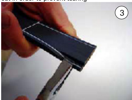
After scratching, tear open the edges from the front using a pair of pliers.
