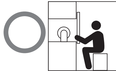
While working, a person is inside the sensor's detection zone.
