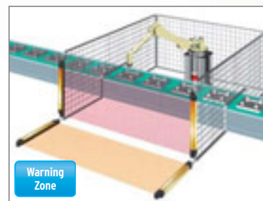
Dividing the zone between series-connected sensors
