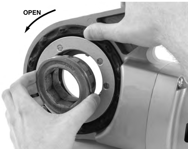
Figure 8 – Installing Adapter Into 690-I
