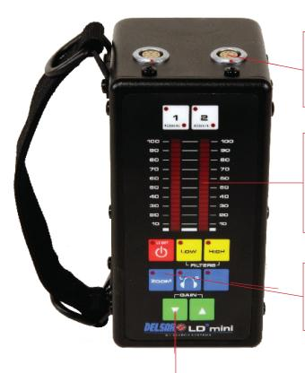
Dual inputs for increased sensor deployment flexibility. Allows two acoustic search probes to be used simultaneously for stereo comparison.
