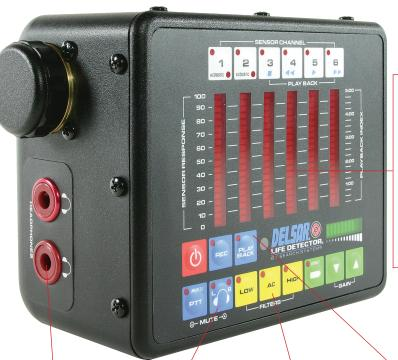
Display panel shows relative signal strength of all six sensors simultaneously to allow positive identification of the strongest signal. Peaking meter on each bar indicates highest amplitude reached by each sensor.
