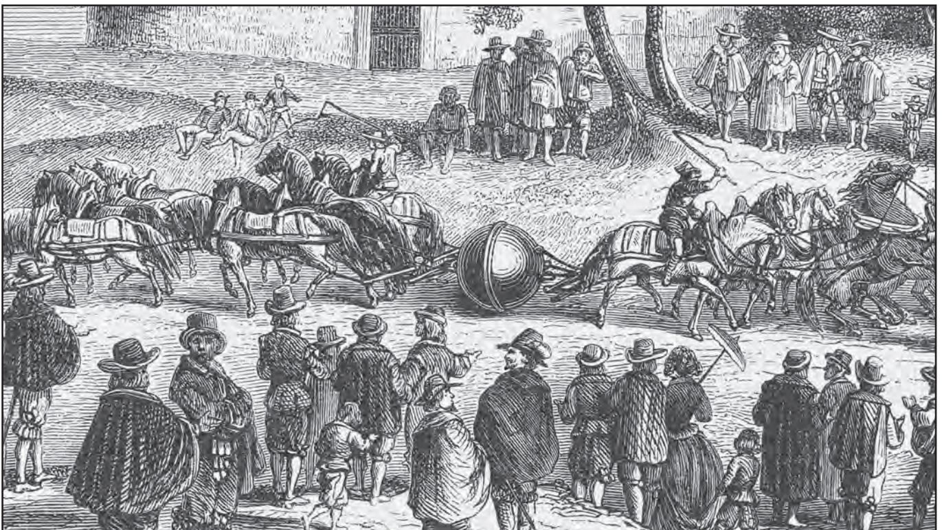
In the "Magdeburg hemispheres" experiment by Otto von Guericke in 1657, the air in the sphere was removed using a pump so that there was no longer any air pressure inside the sphere (vacuum). The outside air pressure pushed the hemispheres together so strongly that they could not even be separated using the pulling force of 16 horses.
