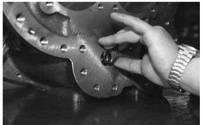
Fig. 3-63 “O” Rings of Vi Adjusting Rod
