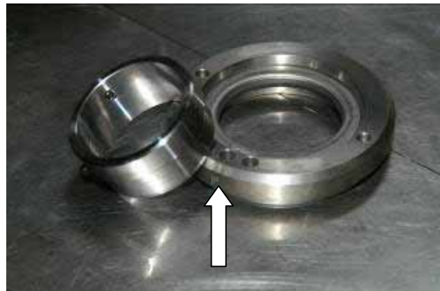
Fig. 3-118 Notch in Seal Retainer
