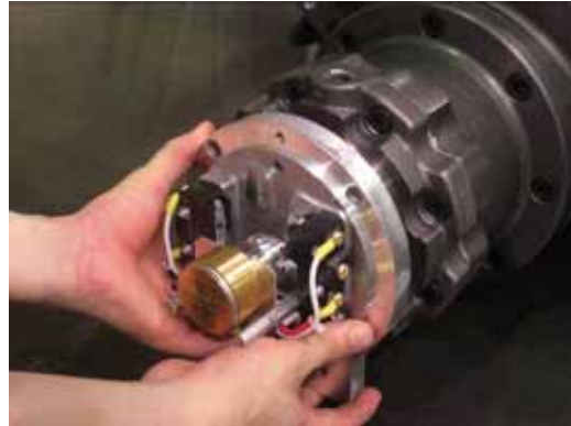
Fig. 3-18 Removing the Micro-switch Base Plate
