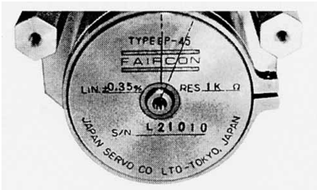
Fig. 3-130 Positioning Mark on Potentiometer
