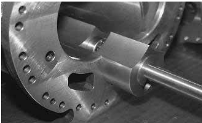
Fig. 3-60 Pulling Out the Variable Vi Auxiliary Valve and Unloader Slide Valve
