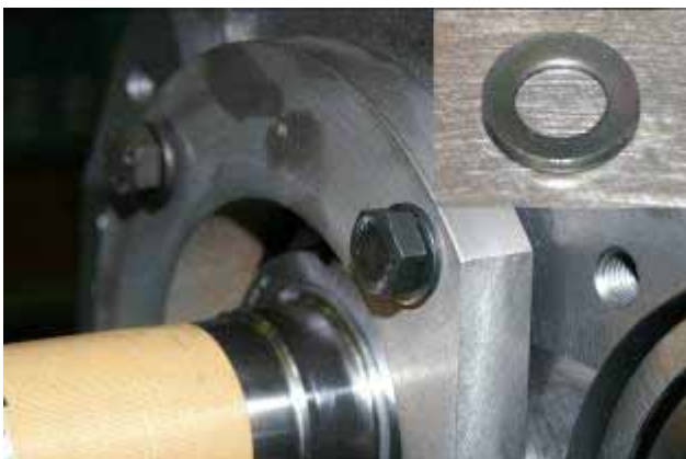
Fig. 3-42 Removing the Thrust Bearing Glands (1)
