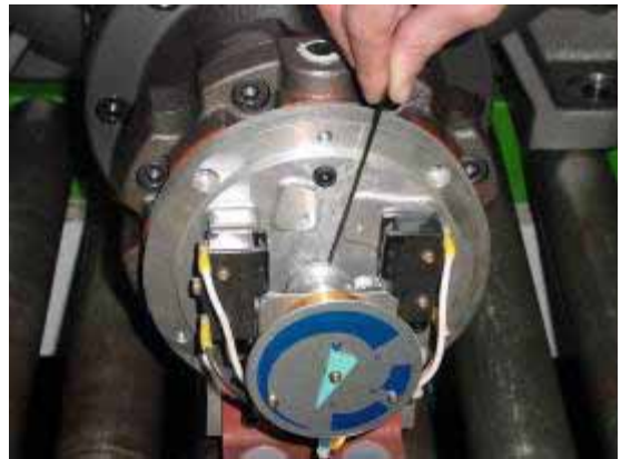
Fig. 3-16 Loosening the Micro-switch Cam Screws
