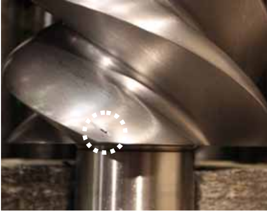
Fig. 3-74 Stamp Mark on Suction Side Lobe End of Male Rotor
