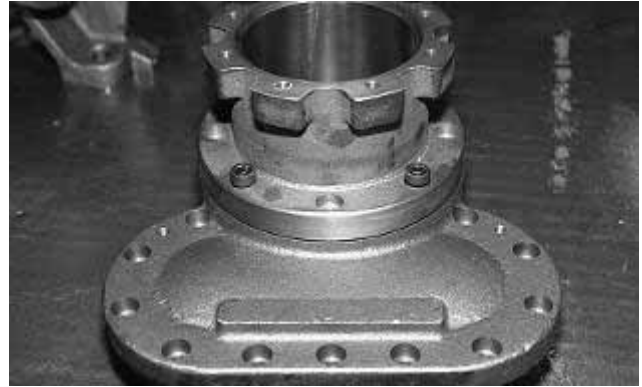
Fig. 3-109 Installing the Unloader cylinder on Balance Piston Cover
