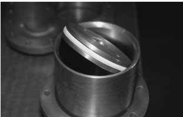
Fig. 3-106 Unloader Cylinder and Unloader Piston
