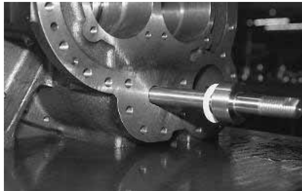
Fig. 3-59 Pulling Out the Vi Adjusting Rod
