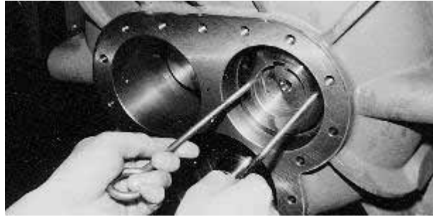
Fig. 3-32 Pulling Out the Balance Piston
