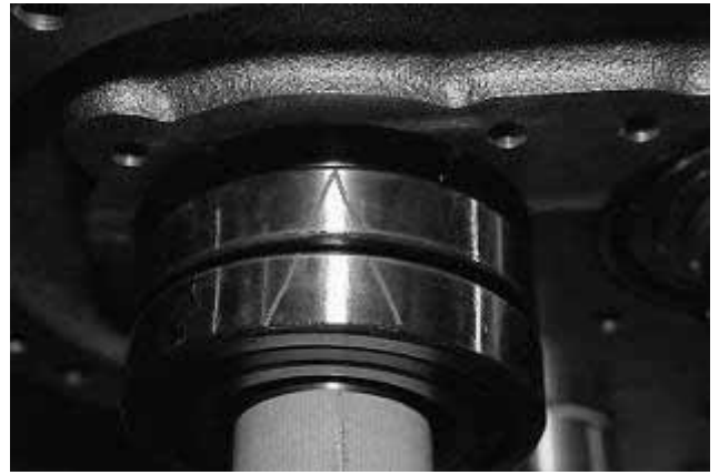
Fig. 3-89 V Mark on Thrust Bearing
