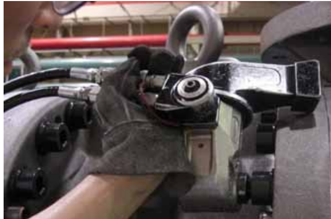
Fig. 3-87 Tightening the Screws with Hydraulic Torque Wrench – Large-sized Models
