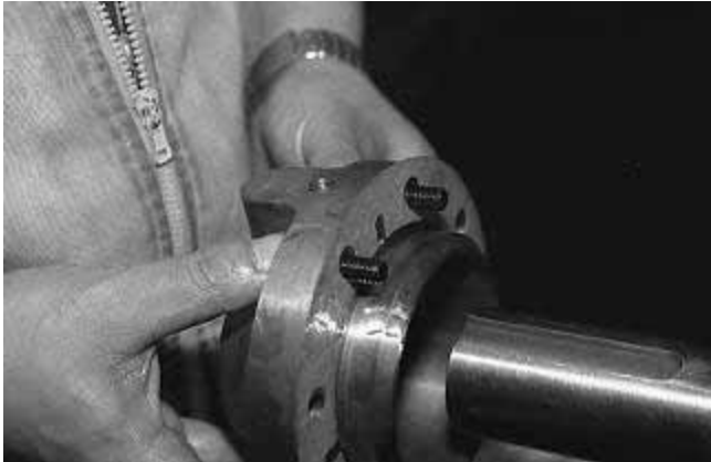
Fig. 3-123 Installing the Seal Cover
