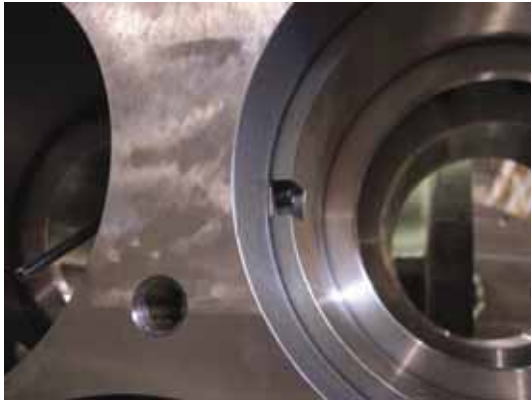
Fig. 3-33 Balance Piston Locking – Type 1
