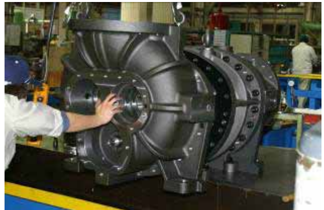
Fig. 3-83 Assembling the Suction Cover with Main Rotor Casing (Using a Crane)
