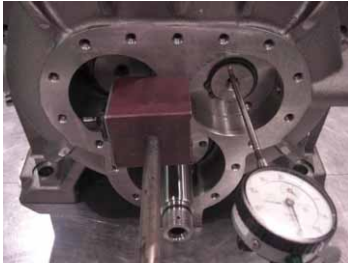
Fig. 3-95 Measuring the End Clearance
