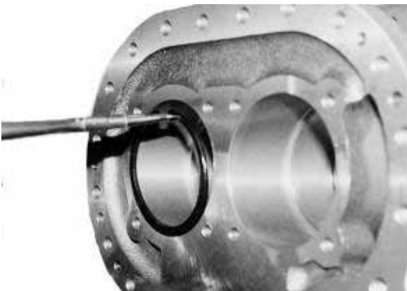
Fig. 3-62 Removing the Stop Ring
