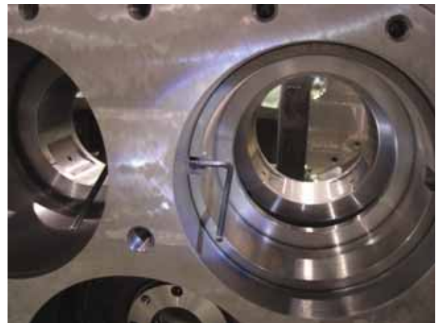
Fig. 3-35 Loosening the Balance Piston Locking Screw
