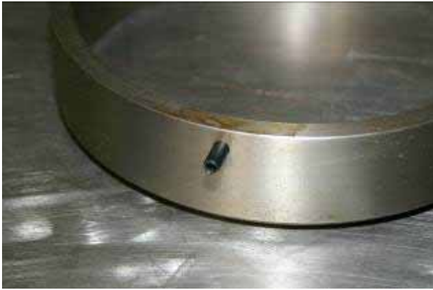
Fig. 3-36 Spring Pin for Locking the Sleeve – 320V
