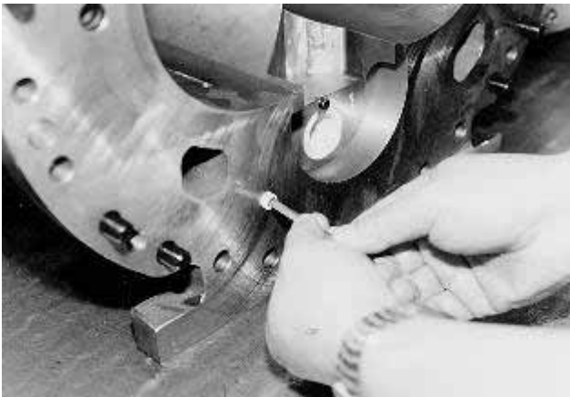
Fig. 3-68 Plug of Oil Injection Circuit Hole (1)
