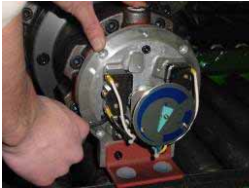
Fig. 3-17 Removing the Micro-switch Base Plate Screws
