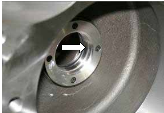
Fig. 3-81 “O” Ring and “O” Ring Gland (P/N 326)
