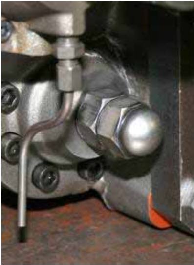
Fig. 3-38 Removing the Vi Adjusting Rod Lock Nut
