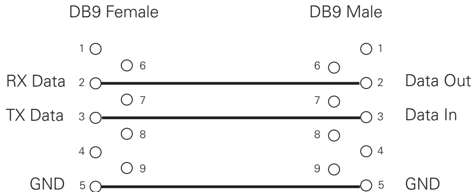
FIGURE 14-3. RS232 extension cable/connector wiring diagram
