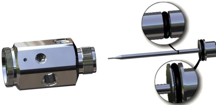
6. Remove needle [70] by pushing the needle upwards from the front of the body [10] until the piston clears the back of the nozzle body, here the piston can be held and the complete assembly can be withdrawn. Check the both O-Rings [71 + 72] of the needle for any damages and replace them, if necessary.
