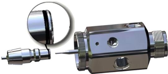
5. Withdraw liquid insert [20] by hand. Check the O-Ring [21] of the liquid insert for any damages and replace it, if necessary.
