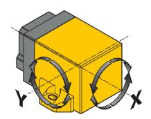
The sensor is able to display any angular value via 2 axes. The drawing shows the assignment to the respective inclination axes X or Y.
