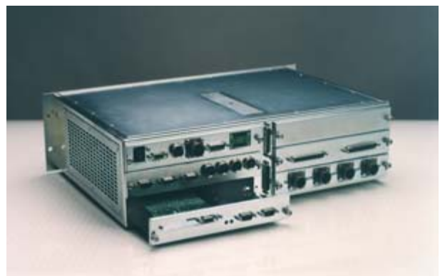
Integrated mainframe 6 slots - 19" - 3HE
