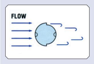
The differential pressure developed across the Flo-Bar is proportional to the square of the flow velocity, and can be measured using either a DP cell, a simple mechanical pressure gauge, or even displayed on a liquid U-tube manometer – depending on the application requirement. The Flo-Bar is available with a number of standard options. Particularly useful is the integral three valve manifold.
