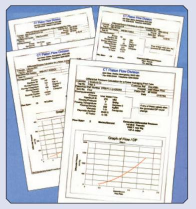
Site data required to produce a Flo-Bar calculation sheet includes fluid type, temperature and pressure, normal flow rate or required flow range, pipework internal dimensions and pipe wall thickness.
