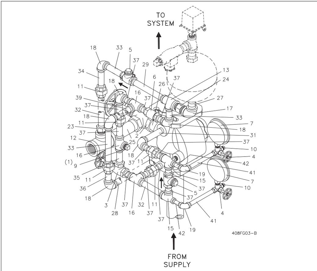
(1) This plug may be removed to install a non-silencable alarm pressure switch.
