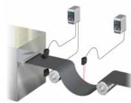
Thickness measurement/loop control of a rubber sheet
