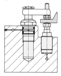
Support and clamping forces have to be adapted to each other, so that there will be sufficient force reserve available for the threaded-body work support to absorb the machining forces.
