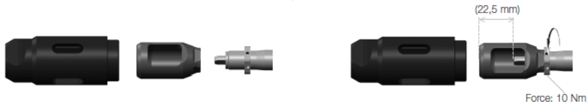
Figure 3 - Fork and nose for studs & force >18 kN (M8 & M10)
