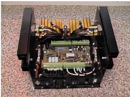
The battery charger fully conforms to NFPA number 20 and will recharge a fully discharged battery within 24 hours.
