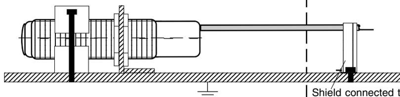
Shield connected to PE large-surfaced
