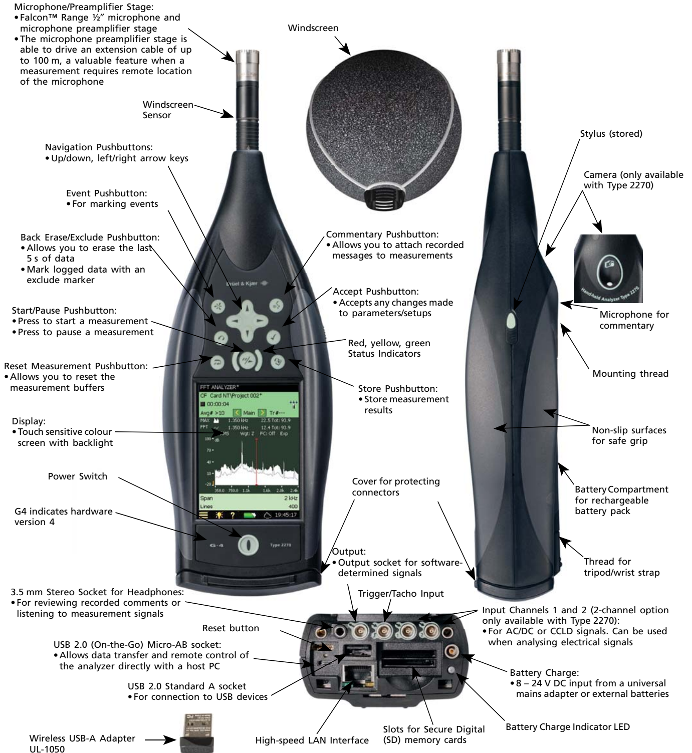
Fig. 1 Key features of Hand-held Analyzer Types 2250 and 2270
