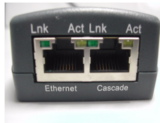
Figure 3-5 Spider RJ45 Ethernet and Cascade Ports
