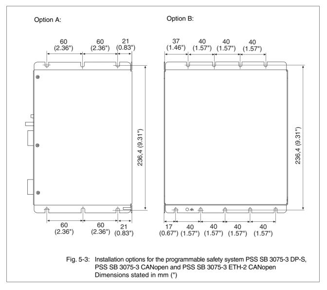
Dimensions in mm (") excluding interfaces and operating controls : H x W x D: 246.4 x 196.8 x 162 (9.70" x 7.58" x 6.38")
