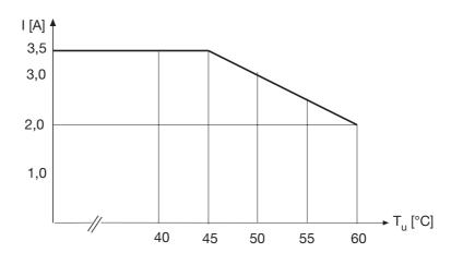
Max. current load capacity of 3.5 A when T  $_{\rm u}$  >45 °C Continuous duty: 60% based on T  $_{\rm max}$ : 40 s
