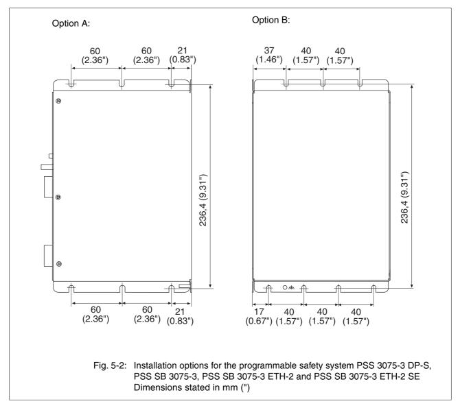
Dimensions in mm (") excluding interfaces and operating controls : H x W x D: 246.4 x 160.2 x 162 (9.70" x 6.31" x 6.38")
