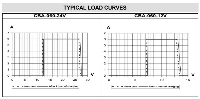
Measures in accordance with CEI-EN60335-2-29 Continuous line = initial characteristic Broken line = work characteristic
